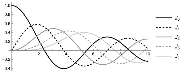
FIGURE 2. Bessel functions of the first kind
