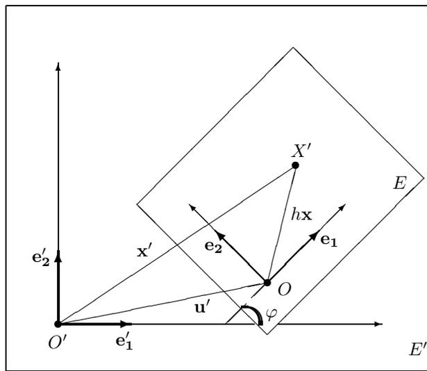
Figure 1. The moving and the fixed planes
